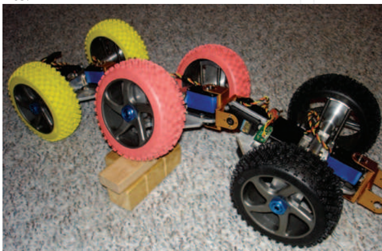
Fig. 15. Proof-of-concept prototype of Wheeler – 3 segments (out of planned 7 segments) connected with 2 DOF joints
