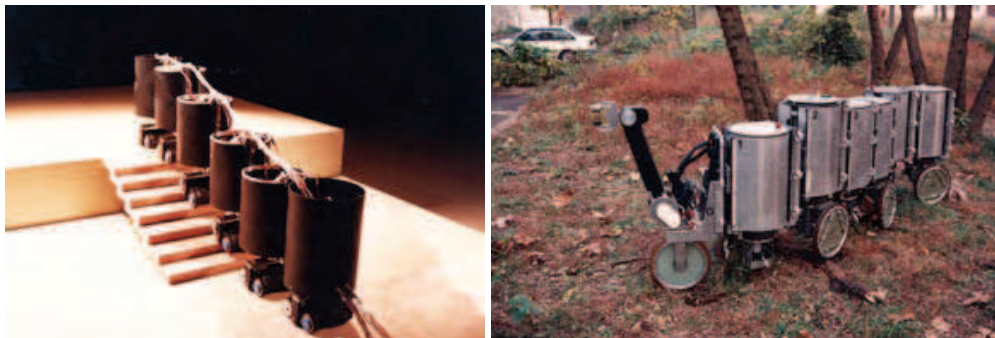
Fig. 3. The Koryu-I (KR-I) robot on the left and KR-II on the right (reproduced from http://www-robot.mes.titech.ac.jp )
