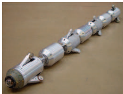
Fig. 10. Pipeline Explorer from NREC (reproduced from http://www.rec.ri.cmu.edu/projects/explorer )
