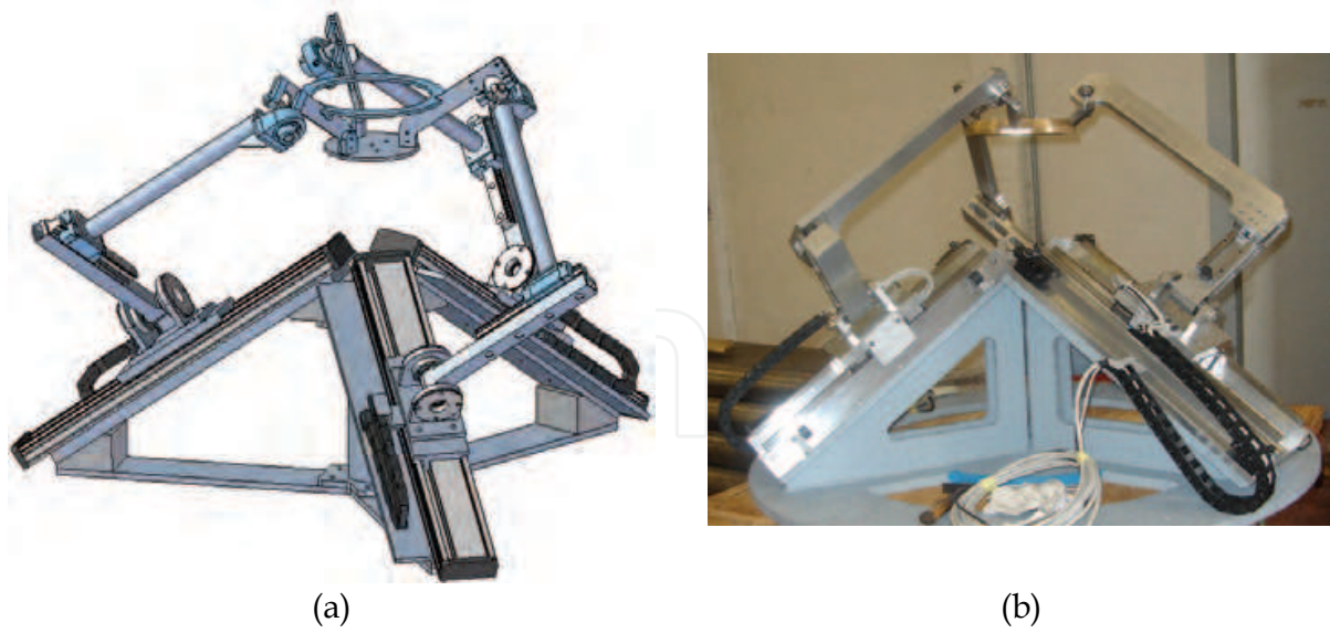
Fig. 26. CAD model of spherical wrist (a) and picture of first laboratory prototype (b)
