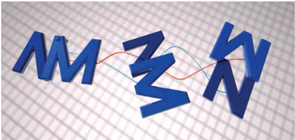
Figure 6: Snapshots of the free flying NM-logo. The two curves correspond to the trajectories of the mass centers of the individual bodies constituting the present multibody system ( t \in \{0, 1, 2\} s).
