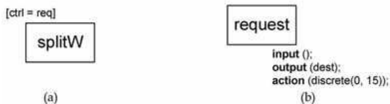
Fig. 5. Transitions with guard condition (a) and transfer function (b)
