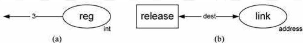
Fig. 6. Unidirectional arc with mapping to value 3 (a), bidirectional arc with mapping to variable dest (b)
