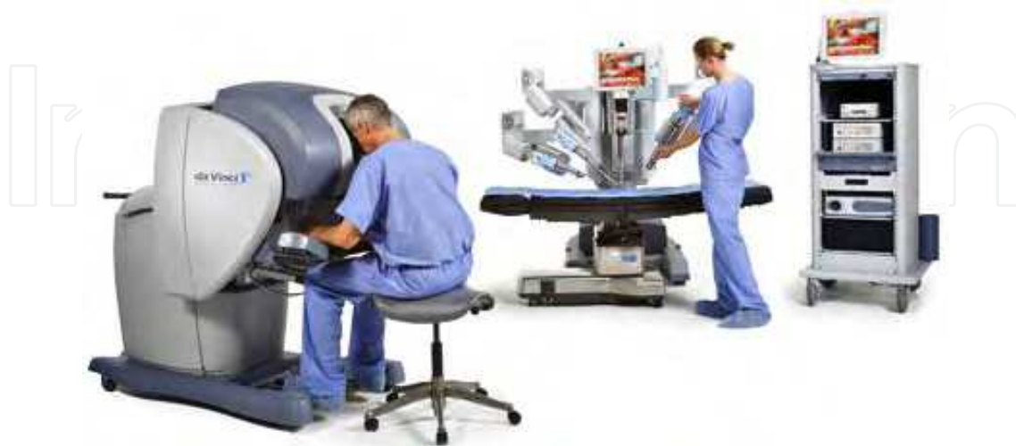
Figure 1. da Vinci system®. It consists of a surgeon's console, a patient-side cart with three or four interactive robotic arms, a high-performance InSite ® Vision System and proprietary EndoWrist ® Instruments
