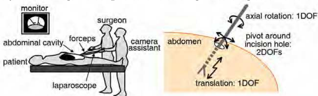
Figure 1. Laparoscopic surgery; surgeon manipulates forceps watching video from laparoscope controlled by camera assistant (left). Limitation of degrees of freedom (rotation, translation, and pivot) is one of causes that make laparoscopic surgery difficult for surgeon (right)
