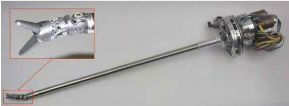
Figure 6. General view of the DLR MIRS instrument and detailed view of its distal end
