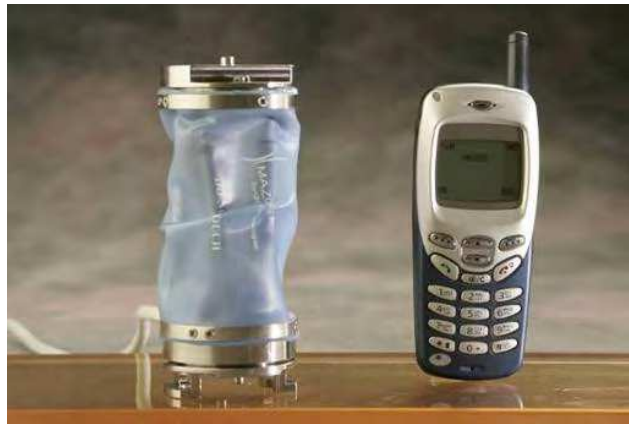
Figure 1. The SpineAssist miniature robot
