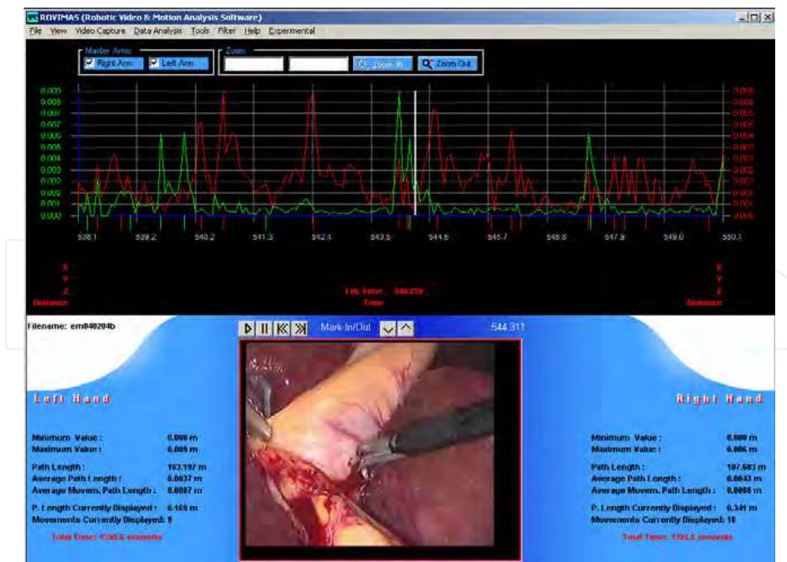
Figure 2. Sample screen image of surgical video synchronized with motion analysis graphics and data. Published with authorization of the Revista Colombiana de Cirugía
