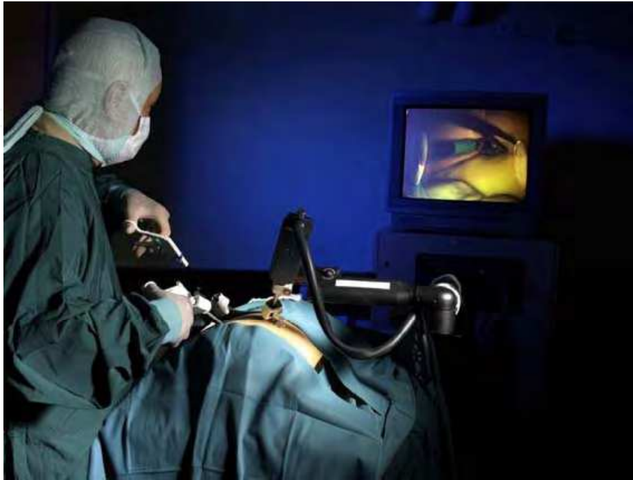
Figure 8. DLR automated camera guidance scenario with AESOP robot
