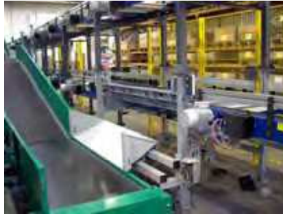
Figure 8. A discharger element that can tilt the tote, so bags slide onto the conveyor belt
