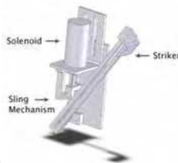
Figure 3. The right arm striking mechanism
