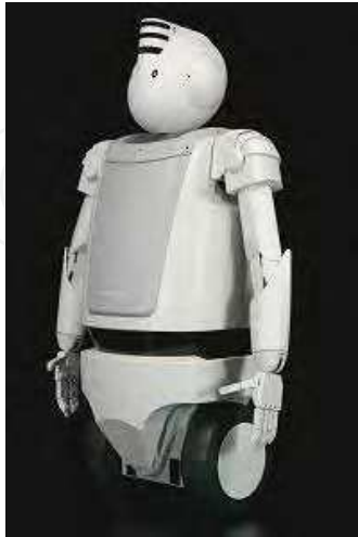
Figure 1. Appearance of EMIEW: body height is about 130cm. maximum speed is about 6 km/h. EMIEW has 8 microphones around his ears and neck. EMIEW is able to communicate with people even under noisy environment
