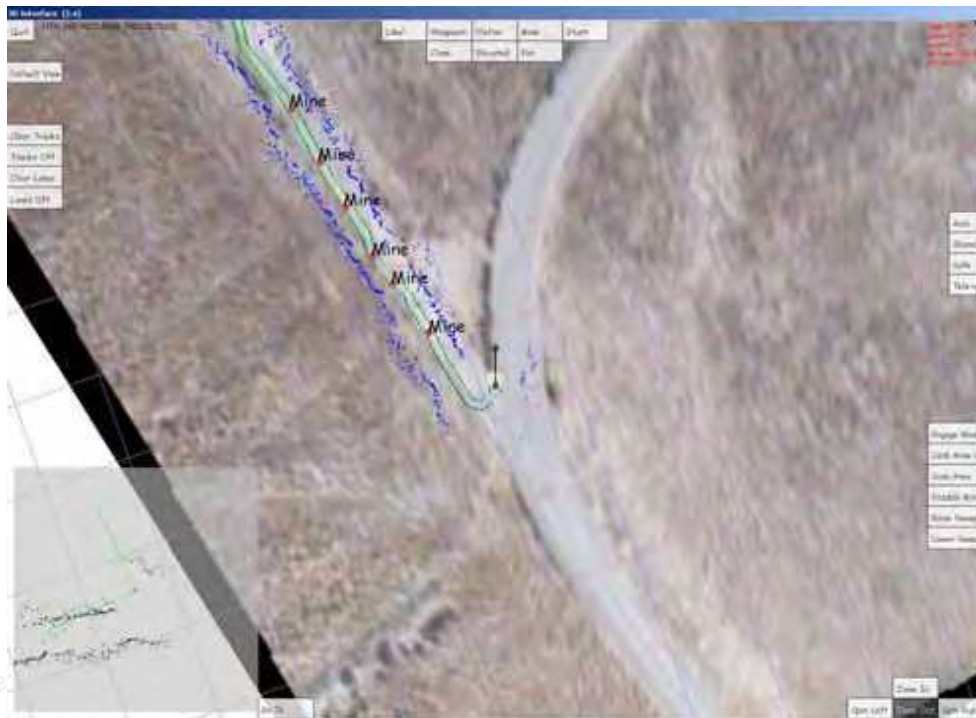
Figure 6. Interface showing fused robot map and mosaiced real-time aerial imagery during a UAV-UGV mine detection task
