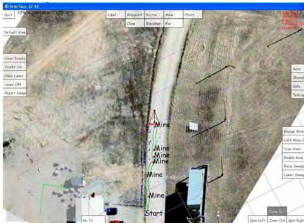
Figure 11. Interface shows the operator the position of mines detected along a road
