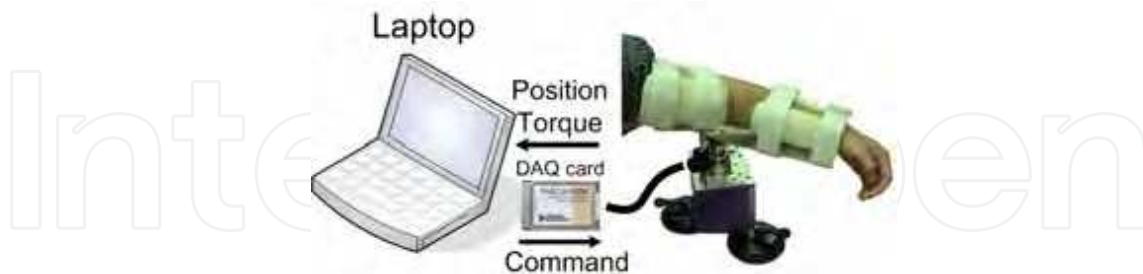
Fig. 2. Control diagram of the limb-stretching device: The device was controlled by a laptop for portability.
