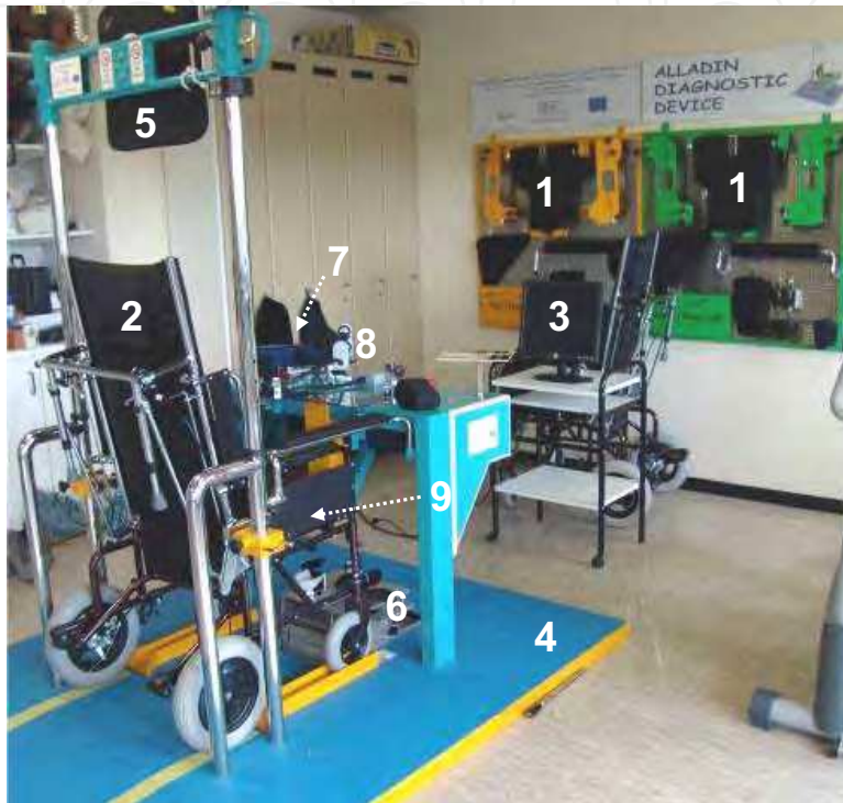
Fig. 2. The components of the Alladin diagnostic device.
