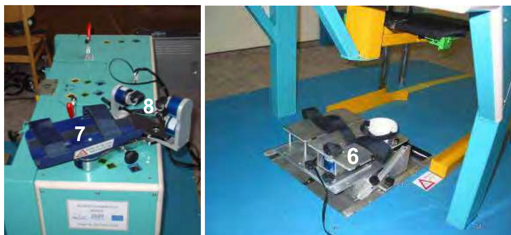
Fig. 3. Devices for measurements on the upper limbs and lower limbs. Left: the Arm Device (7) and the Finger Device (8). Right: the Foot Device (6).
