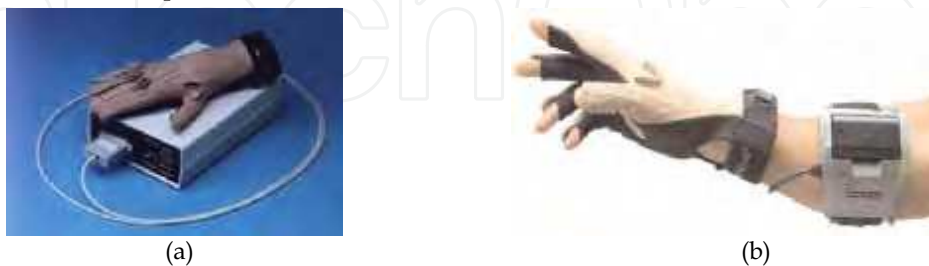
Fig. 3.3. The Cyberglove sensing Glove (a) Desktop version (b) Bluetooth wireless version. Picture Immersion Corporation.
