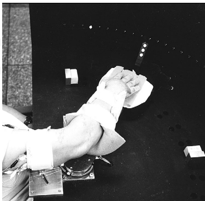
Fig. 2.5. Robotic Assistance of Upper Limb Exercise. The image depicts the orthoses, the contact points with the arm and the target towards which the lever should be aimed during extension and flexion of the elbow (Cozens, 1999).
