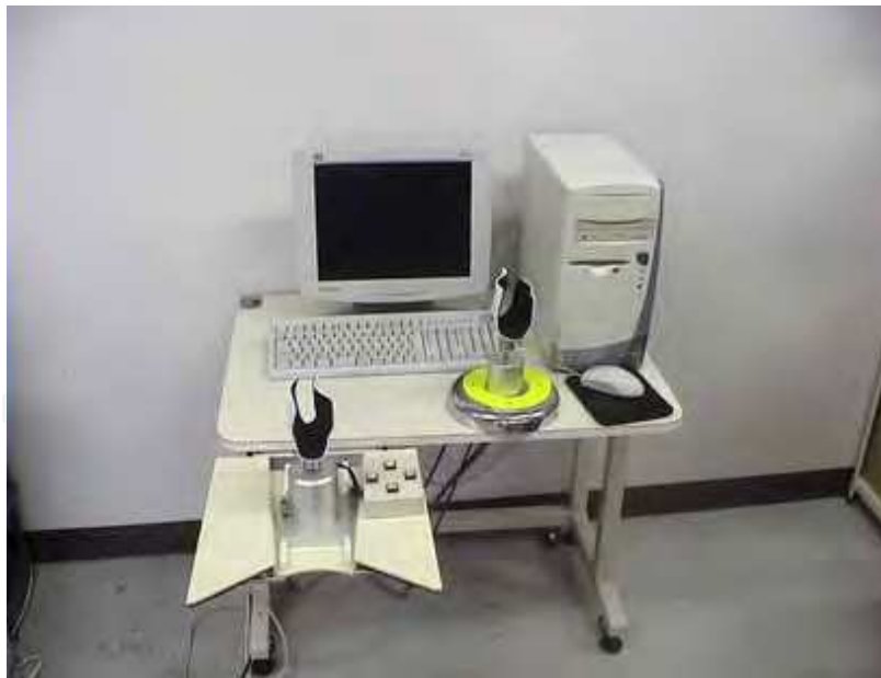
Fig. 1. The first and second prototype of upper limb rehabilitation system for spinal cord and peripheral nerve injury. The first prototype in the front left is mounted on a stage to place on the laptop. The second prototype is for desktop use.
