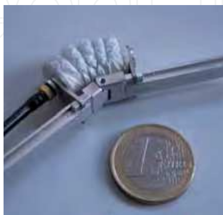
Fig. 2. Flexible fluidic actuator with artificial joint.
