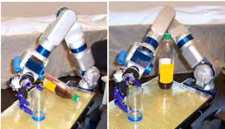
Fig. 17. Example of dexterous manipulation: a 6-joint arm can’t grasp a glass without collision with a bottle (left); by controllable movement of elbow it will be possible (right).
