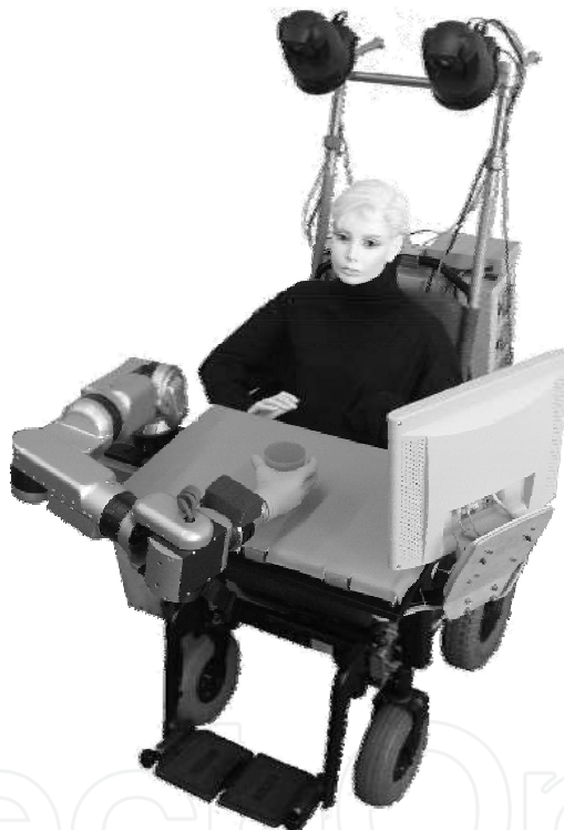
Fig. 3. Rehabilitation robotic system FRIEND-II.
