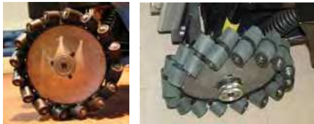
Fig. 15. Mecanum wheel for omni-directional movement.
