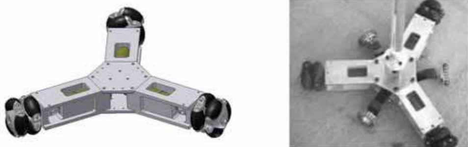
Fig. 4. (a) Three black omni directional poly-roller wheels act as actuators, (b) three free omni directional small-roller wheels used in a feedback mechanism
