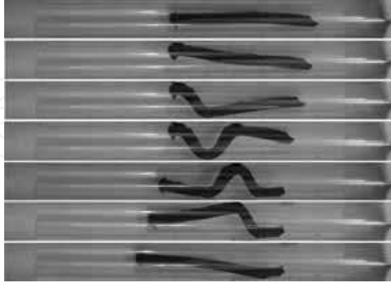
Fig. 17. Magnetizable elastic body (sample 1) in the travelling magnetic field
