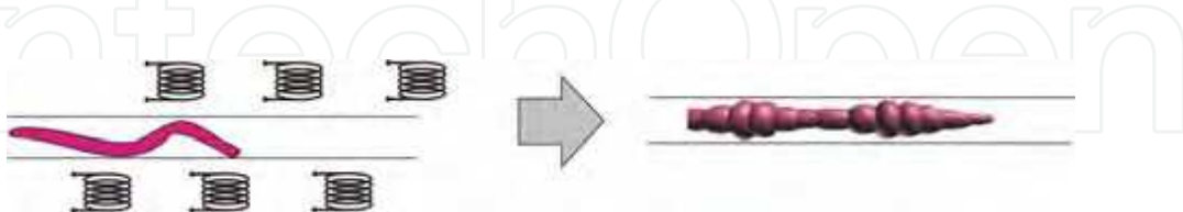
Fig. 28. From the snake-like concertina motion to worm-like peristaltic crawling
