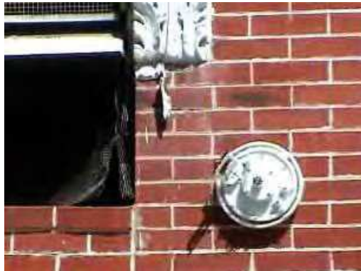
Fig. 13. City-Climber prototype-I approaching a window on brick wall, a CMU-camera is installed on a pan-tilt structure for inspection purpose.
