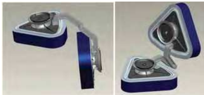
Fig. 15. Two robot modules connecting by a hinge in +90^\circ , and -90^\circ configurations, being able to make wall-to-wall, and wall-to-ceiling transitions
