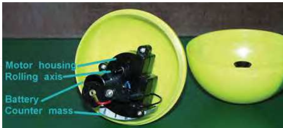
Fig. 8. 'Squiggleball' opened to show the interior parts (Image: TKK)
