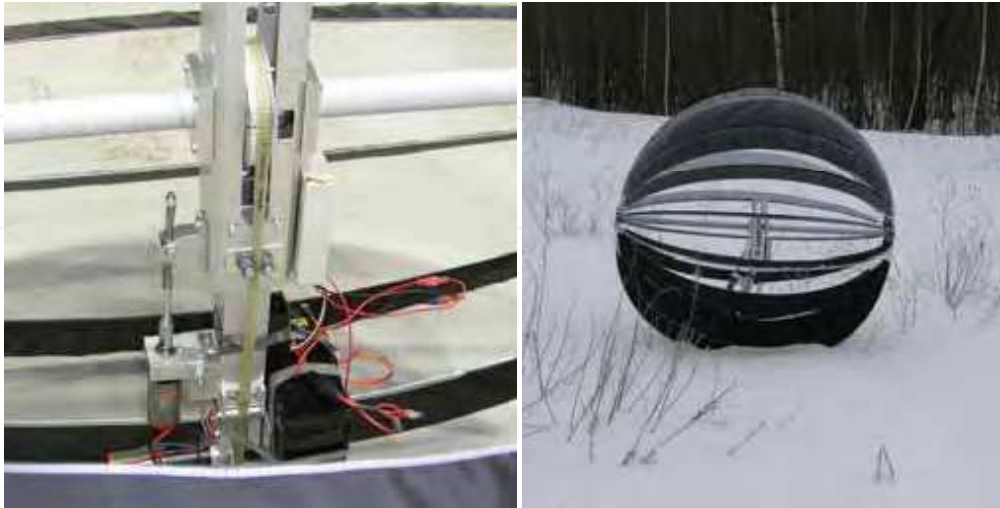
Fig. 18. (left) Thistle mechanism; (right), 1.3-m Thistle rolling on snow bed (TKK)
