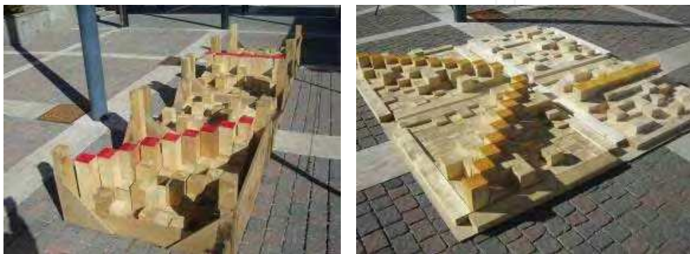
Fig. 2. Step Fields Provide Reproducible Terrain Challenges
