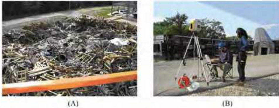
Fig. 14. (A).The wood pile was imaged using three ‘overhead’ scans and several ground-level scans. This view was taken from a scissors-lift. (B) Imaging the train wreck.
