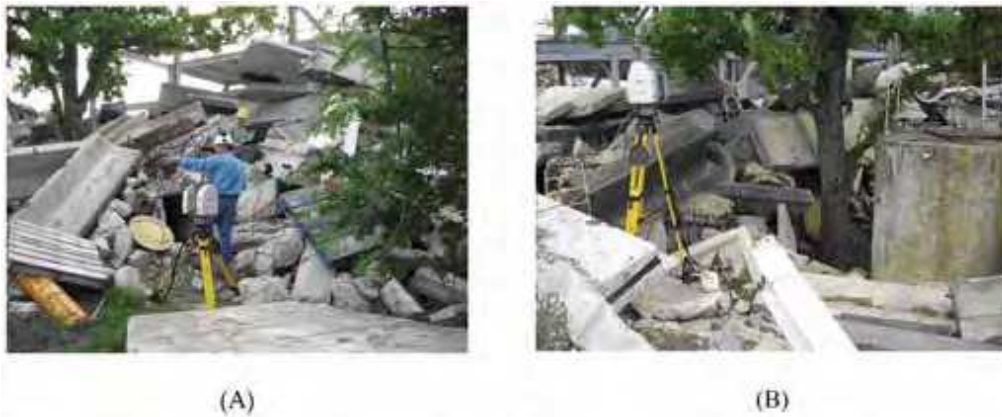
Fig. 13. (A) Setting up a scan of the rubble pile. Scan locations must be carefully chosen to obtain sufficient scene data to capture the existing conditions and enable tie in to prior scans using pre-positioned targets. (B) Since the laser scanner is a line-of-sight device, obtaining sufficient information for a disordered scene such as the rubble pile requires numerous scan locations throughout the environment.
