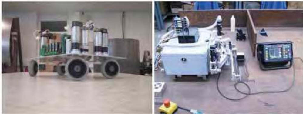
Fig. 15. Left: Platform to test robot motion and trajectory following capability. Right: Fully assembled robot performing NDT on a mock-up with Creep waves
