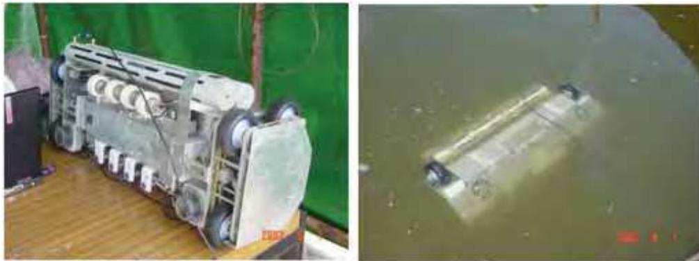
Fig. 5. Left: RobTank with full payload of 4 ultrasonic wheel probes, 4 compression probes and 2 rotating probes; Right: RobTank on the floor of a water storage tank, Sines oil refinery
