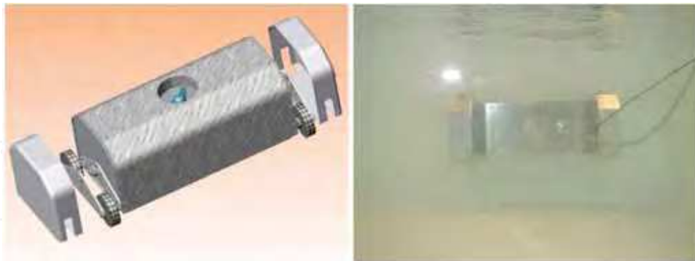
Fig. 2. Left: Solid drawing of RobTank; Right: Vehicle climbing on curved wall (3 metre diameter)
