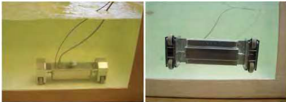
Fig. 1. Left: Robtank immersed in a water tank while inspecting the tank floor; Right: Robot climbing on a glass wall after transition from floor to wall
