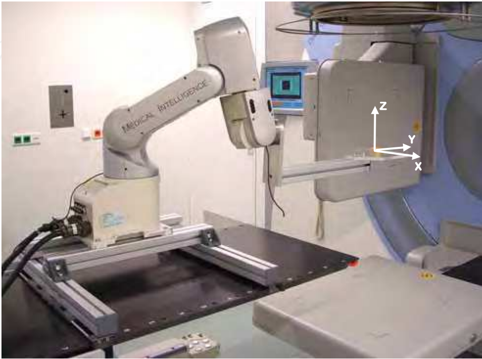
Figure 4. Six-axis robot mounted on the HexaPOD robot table. The gantry head is at the top ( 0^\circ ) and the MV EPID is at the bottom ( 180^\circ ). Attached to the robot is a phantom with a wooden disk on a slab of Plexiglas representing the object to be tracked. Note that for actual treatment of patients a head extension board is attached to the HexaPOD table
