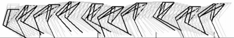
Figure 12. Illustration of a suboptimal gait based on asymmetric jumping. It is similar to the fastest horse gait called gallop
