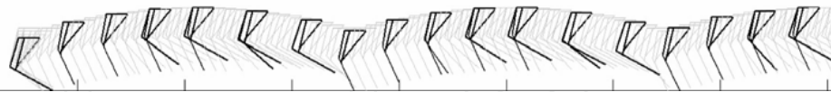
Figure 14. Illustration of the optimal gaits based on jumping. This is the most efficient gait obtained, but in real life this gait has many drawbacks. E.g. the slippery effect in the floor to feet friction when the robot kicks hard
