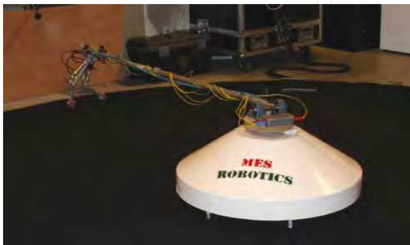
Figure 2. The entire system containing the robot, the balancing rod and the hub
