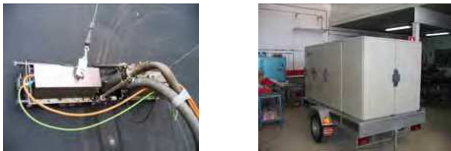
Figure 6. Lázaro II and portable control unit with enough space to place the robot inside
