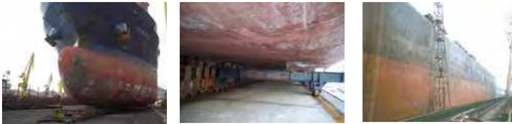
Figure 2. Different requirements for the cleaning devices: bow, bottoms and vertical surfaces
