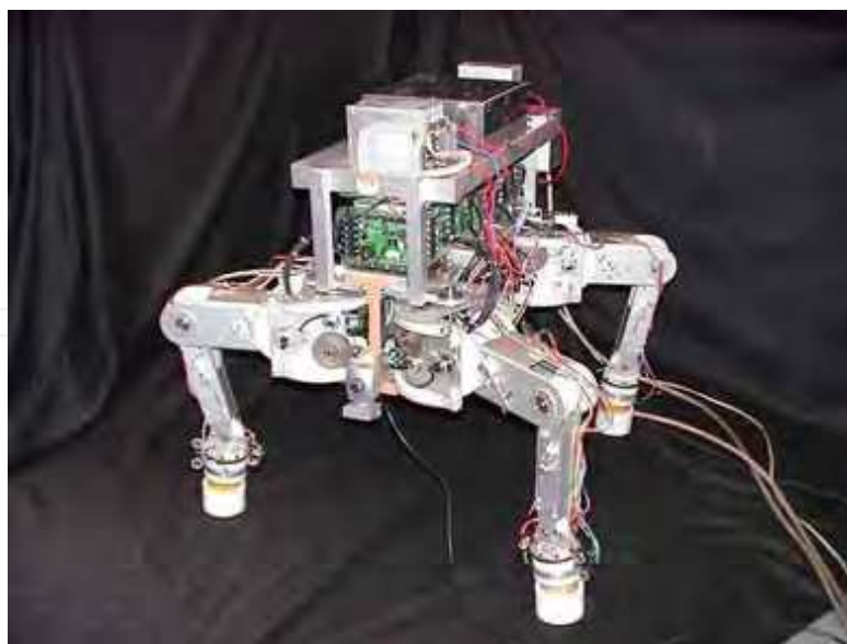
(a) TITAN-VIII with the integrated sensors
