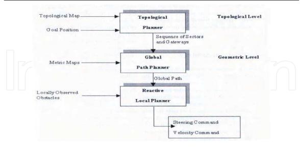
Figure 6. Three – level path planning and navigation.
