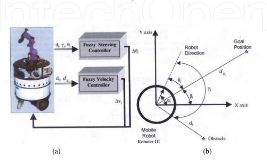
Figure 3. (a) The Robosoft Robuter III mobile robot of IRAL / NTUA connected to the corresponding fuzzy-based obstacle avoidance unit.
