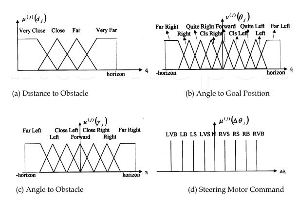
Fig. 4. Fuzzy sets for the mobile robot: (a) distance to obstacle, (b) angle between robot and goal position, (c) angle between robot and obstacle, and (d) steering motor command. Note that the output is not partitioned into fuzzy sets, but consists of crisp values.
