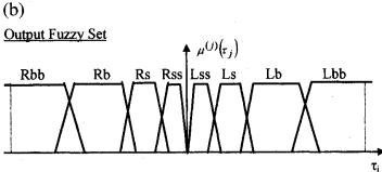
Figure 2. Repeller, attractor and output fuzzy sets for link 2.
