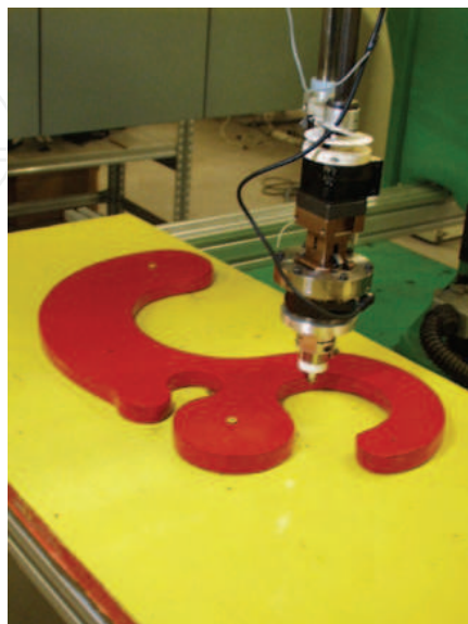
Figure 1. The SCARA robot during the contour tracking of a complex shape
