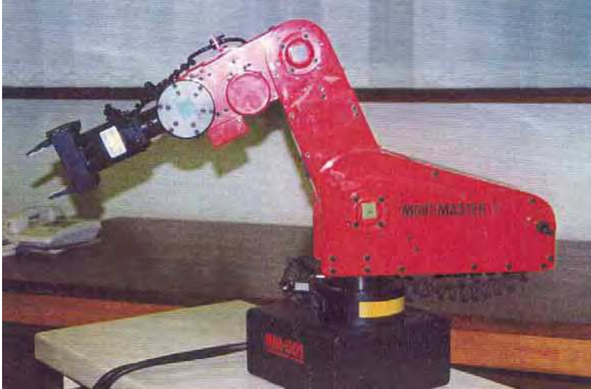
Figure 8. The Mitsubishi RM-501 Move Master II Industrial Robot.
