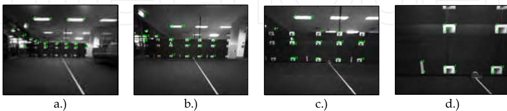
Figure 4. Rectified images overlaid with features at (a) 5.4 m (b) 3.9 m (c) 2.4 m (d) 0.9 m
