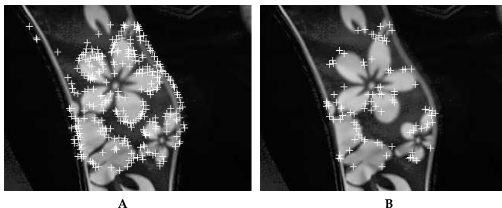
Figure 8. Corner-based scene keypoints (A) and 90^\circ T-junction-based scene keypoints (B) detected in the image from Figure 6. Scanning window radii are 7 and 10 pixels
