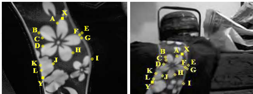
Figure 12. Matched keypoints in the model and test images (⊕ corner keypoints, ■ 90° T-junction keypoints)
