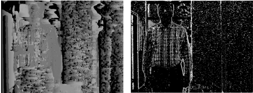
Figure 23. Left: Disparity map. Right: Resulting depth map (in image coordinates)
