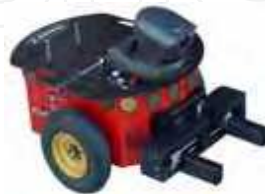
Figure 5. Pioneer 2/DX mobile robot, equipped with a color CCD camera and sixteen sonar sensors around
