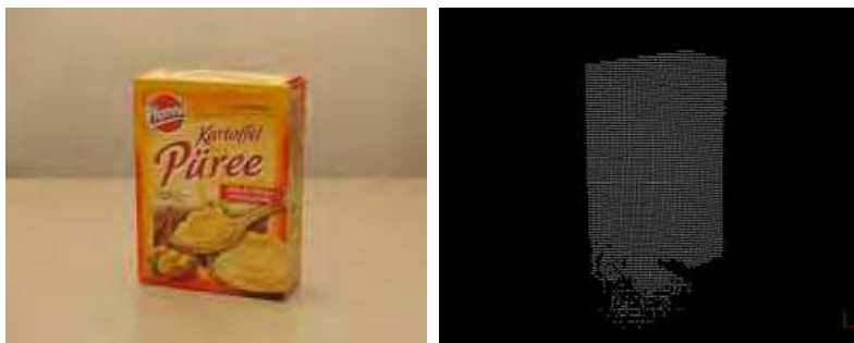
Figure 13. An instant mashed potatoes box. Because of the symmetry plains of the cuboid shape the pose determination gives a set of possible poses. Left: Colour image from a digital camera. Right: 3D range image from the Swissranger SR-2
