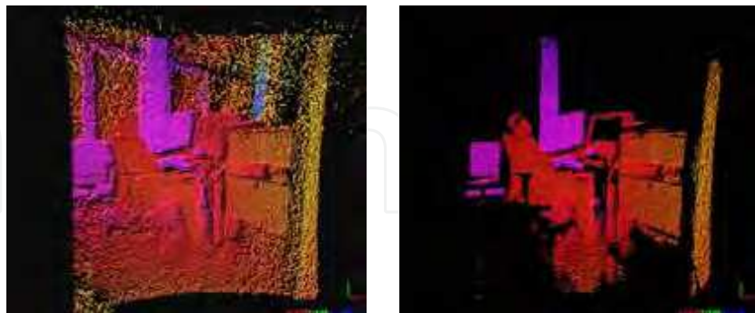
Figure 9. Two images taken with a SwissRanger SR-2 device of the same scene. Left image: without filtering. Right image: with accuracy filter. Only data points with an accuracy better than 50mm are remaining
