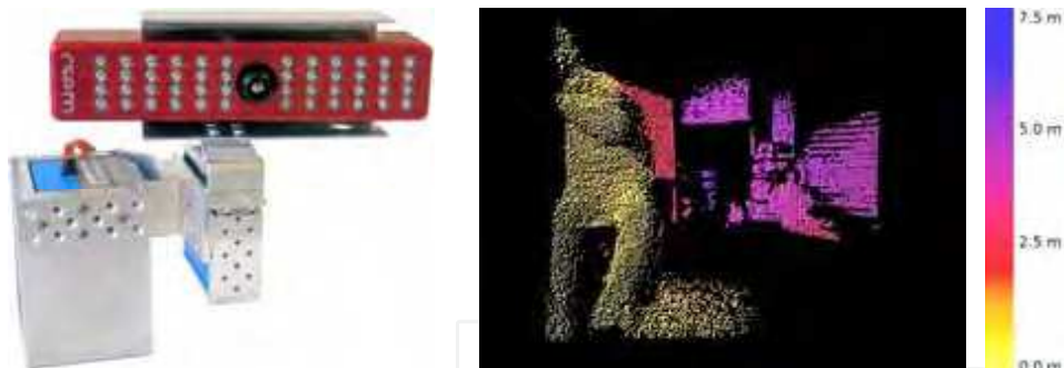
Figure 5. Left image: SwissRanger SR-2 device mounted on a pan-tilt unit. Right image: Sample image captured from a SwissRanger SR-2 device. The image is color coded (see color bar on the right side)
