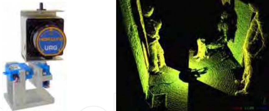
Figure 4. Left image: Hokuyo 3D Scanner. Right image: Scan taken with the Hokuyo 3D Scanner. Note that a field of view of 248° is reached by only one rotating servo
