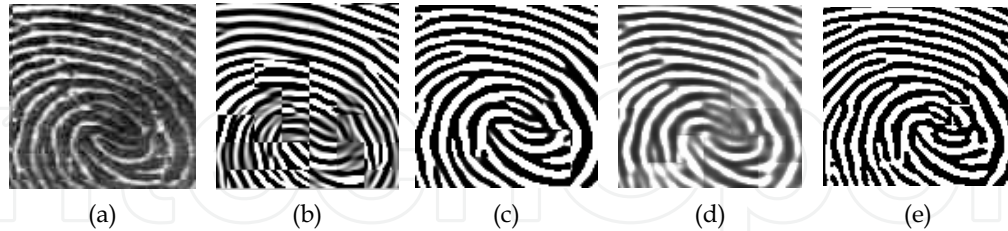
Fig. 10. Example of enhancement results of fingerprint image region with a singular point (core). Original image (a); enhanced image after applying the Gabor-based filter (b), the modified Gabor-based filter(c), the structure-adaptive anisotropic filter (d) and the proposed unique structure-adaptive anisotropic filter (e)
