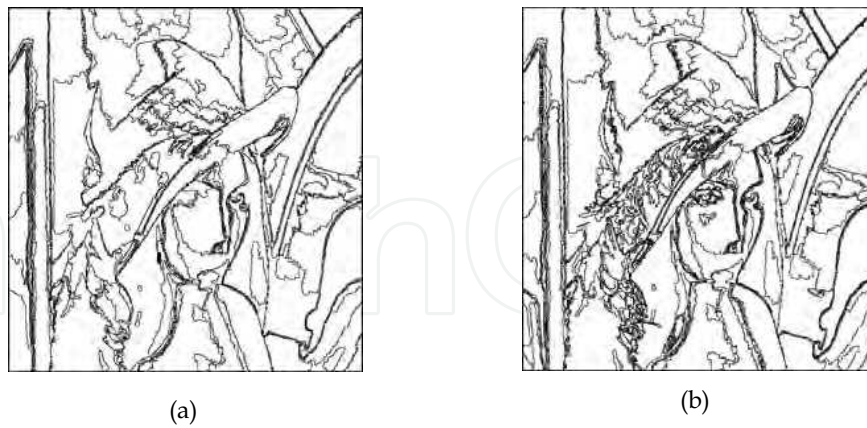
Fig. 7: Oversegmented image created using four partial segmentations of the image Lena: (a) \epsilon = 255 and (b) \epsilon = 50 .
