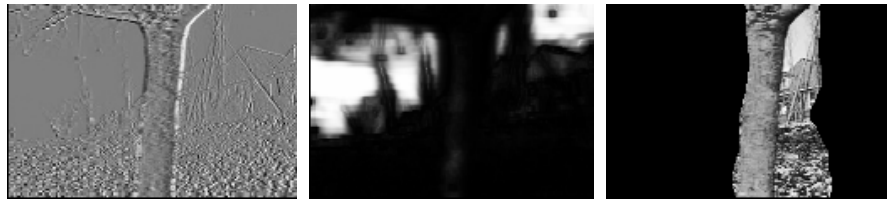
Fig. 9. For the frame in Fig. 7, Left : Inter-frame difference, Centre : Image potential derived from I_t , Right : Segmentation obtained using image potential from image at the centre and initialization with the segmentation from previous frame.
