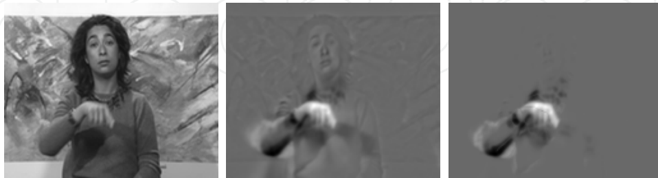
Fig. 3. A frame of the “silent” video sequence: Left : Input data. Centre : Even-symmetric representation of the response of one of the composite features detected, corresponding to the moving hand, calculated using equation (6) and, Right : using equation (7)
