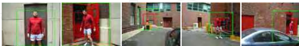
Figure 4. ABCshift successfully tracks throughout the sequence and is not distracted by red regions of background, despite being initialised in image 1 which contains no red background. Frames 1, 176, 735, 1631, and 1862 shown. Green and red squares indicate the search window and estimated object size respectively. This movie, PeopleTracking1ABCshift.avi, can be viewed at the project website (see references).
