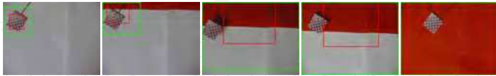
Figure 1. A simple blue and red chequered object, moving from a region of white background into a region of red background. CAMSHIFT fails as soon as the object moves against a background with which it shares a common colour. Frames 350, 360, 380, 400, and 450 shown. Green and red squares indicate the search window and estimated object size respectively. This movie, RedWhite1CAMSHIFT.avi, can be viewed at the project website (see references).
