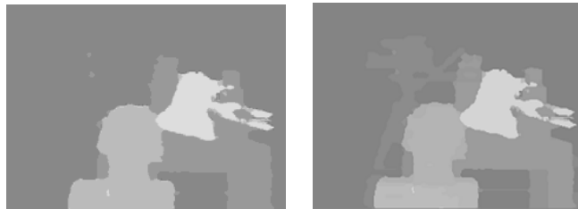
Figure 7. Disparity map after region merging ( tsukuba image) (left: C simulation result, right: VHDL simulation result)
