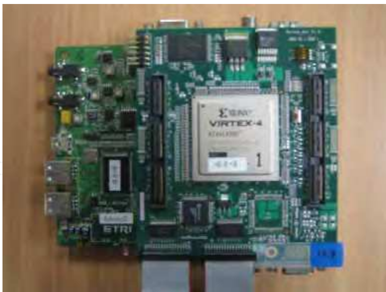
Figure 16. Embedded System and unified FPGA board module
