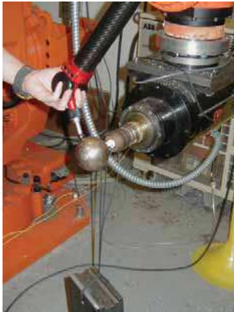
Fig. 15. Experiment Setup for robot stiffness measurement.
