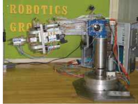
Fig. 2. 6R robot configuration.
