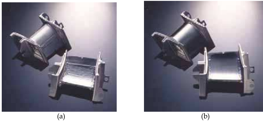
Fig. 18. Vanes before (a) and after (b) robotic grinding and polishing.
