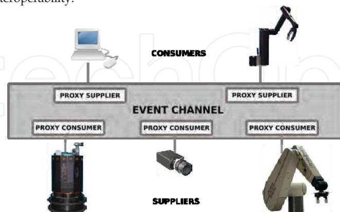
Fig. 5. CORBA Event Service architecture.
