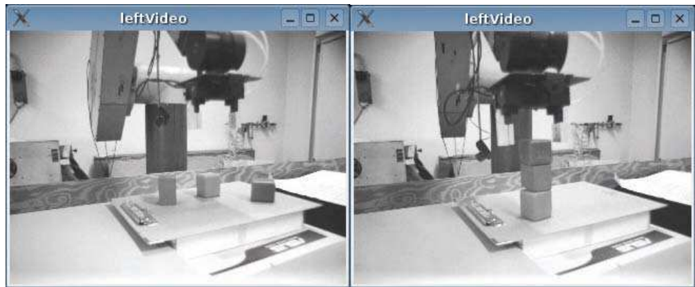
Fig. 13. A stacking experiment with the Puma 560 manipulator. The images are taken from the left eye of the stereo camera.
