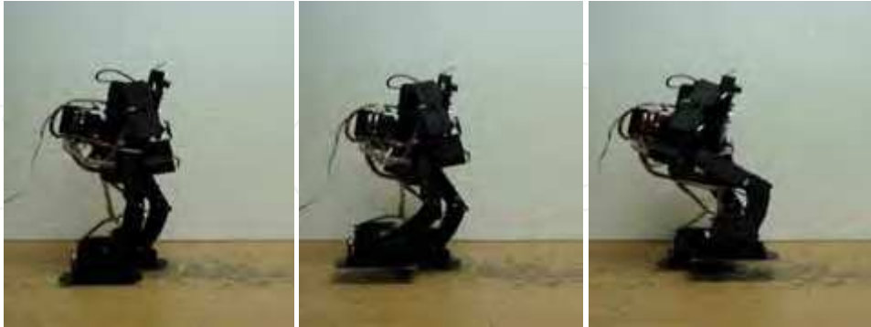
Fig. 18. Side view of the biped humanoid robot on an uneven floor.
