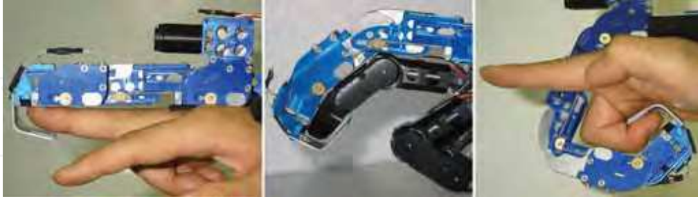
Fig. 26 Master finger mechanism (MAF) following various finger flexions.
